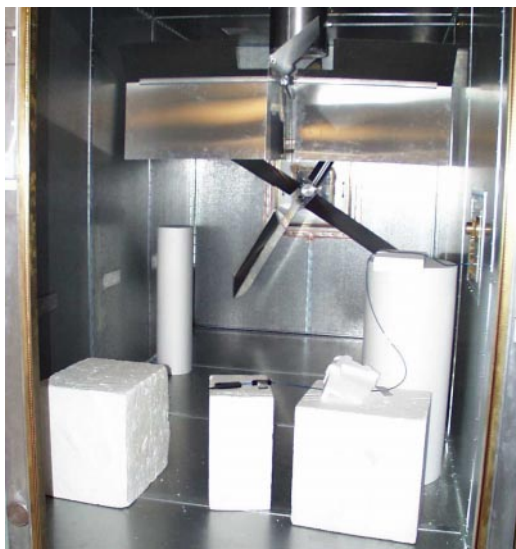
Fig 2: AUT placed inside the E3 RC at FOI.
